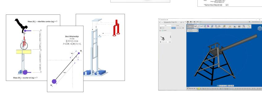
The design phase consisted of calculations for torque, 3D CAD models for the towers, and a spreadsheet for building a new unicycle wheel. Design reviews were held to re-evaluate the design choices as the design matured.
